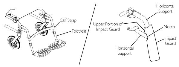
FIGURE 4.6 Installing Impact Guards/Calf Strap
